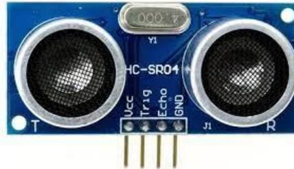
**Gambar 2.** Sensor Ultrasonik HCSR04
