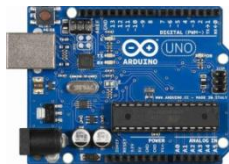
Gambar 2. Arduino UNO (Sumber: www.tokopedia.com )
